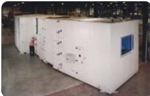
Roof Top Air Handling Unit.
