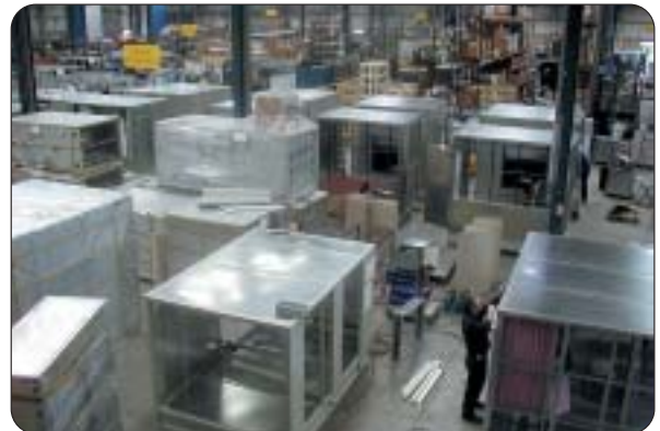
Moducel AHU Production.
