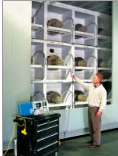
Fan cartridge dynamically balanced.
