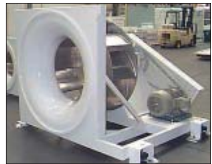
Traditional AHU plenum fan with spring isolation bases.
