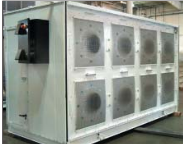
Inlet air straighteners shown.
